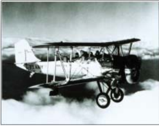
Figure 2: Navy bi-plane with meteorograph on starboard wing strut taking meteorological measurements of pressure, temperature, and humidity.
