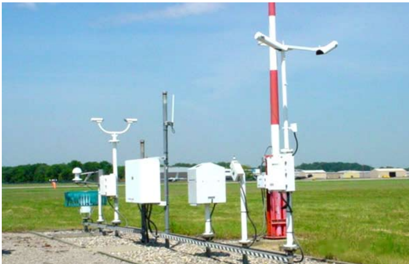
ASOS array from left: precipitation gage, temperature/dewpoint sensor, present weather, data collection package, ceilometer, freezing rain sensor, wind tower, visibility. Photo by NWS Grand Rapids, MI, Electronics Techs Eric Repaal and Thomas Williams.
