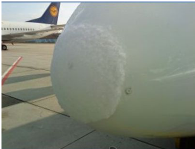
Figure 3: Ice buildup on an aircraft's radome
