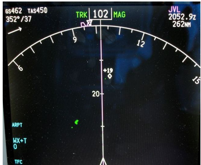
Figure 4: Cockpit weather radar display with the antenna set to auto-tilt too high (0 degrees in this case), showing a small, weak echo in green, to the north (left) of the eastbound aircraft.
