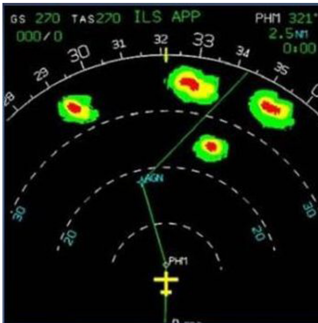
Figure 6: Cockpit weather display showing four strong cells 25-35 miles ahead of the aircraft.
