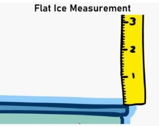
Find a flat surface that has been undisturbed from the surrounding environment or other objects. Measure ice accumulation with a ruler.
