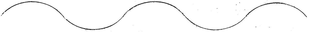
Figure 1a. Longer period waves will develop as the present waves are moving slower than the wind speed ( C < V ). As the wind continues, energy will be added to longer period waves until the waves move as fast as the wind speed.
