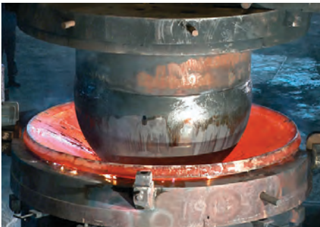
▲ One of the forged hemispheres cools. Material from the hemisphere's interior and exterior was later removed to reduce its thickness to 3 inches.
