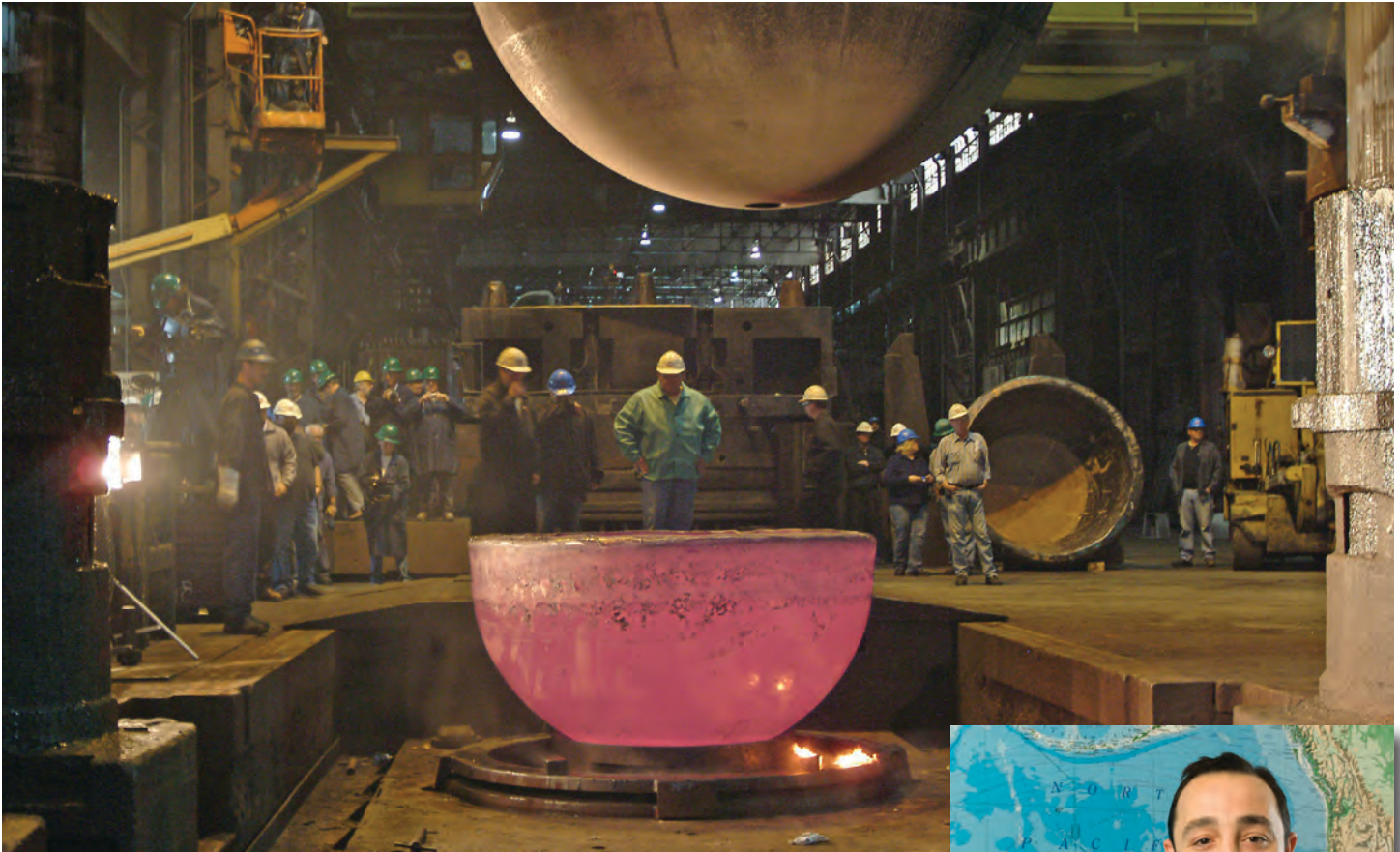
▲ One of the forged hemispheres cools. Material from the hemisphere's interior and exterior was later removed to reduce its thickness to 3 inches.
