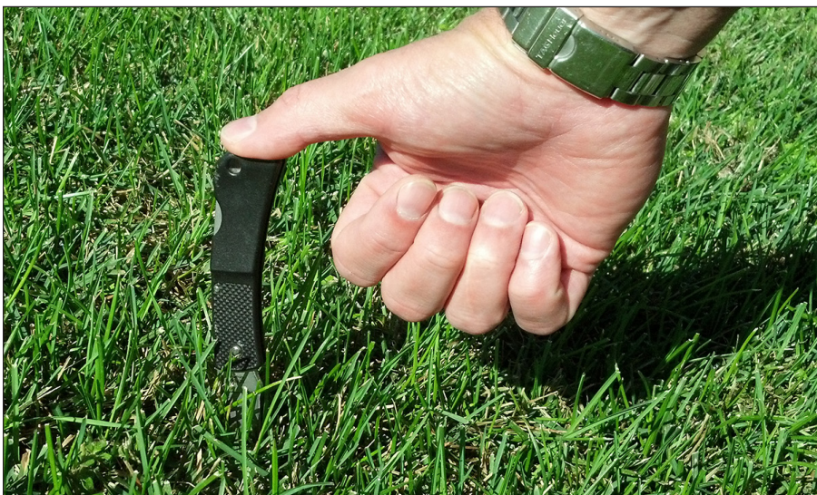
Figure 2. Testing soil compaction with a knife and the force of the thumb.
