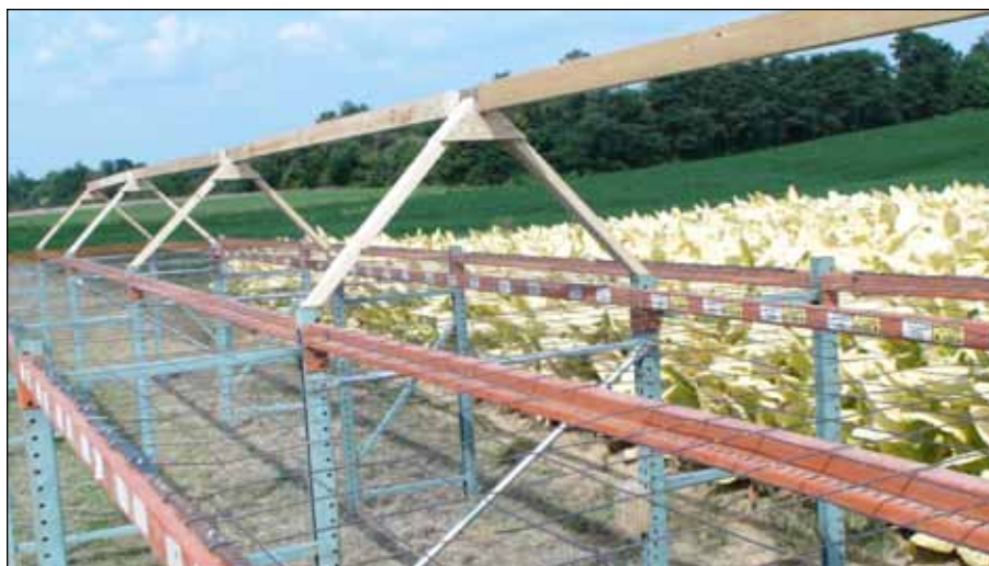
Figure 12. Pallet racks outfitted with wire mesh panels for hanging notched tobacco plants that have been mechanically harvested.
