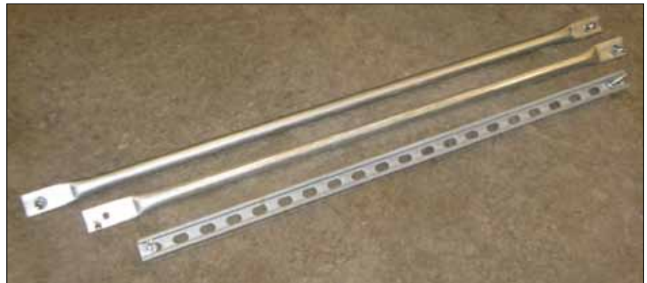
Figure 5. Spacers and braces made out of electrical conduit and standard steel strut C-channel to connect pallet rack sections.
