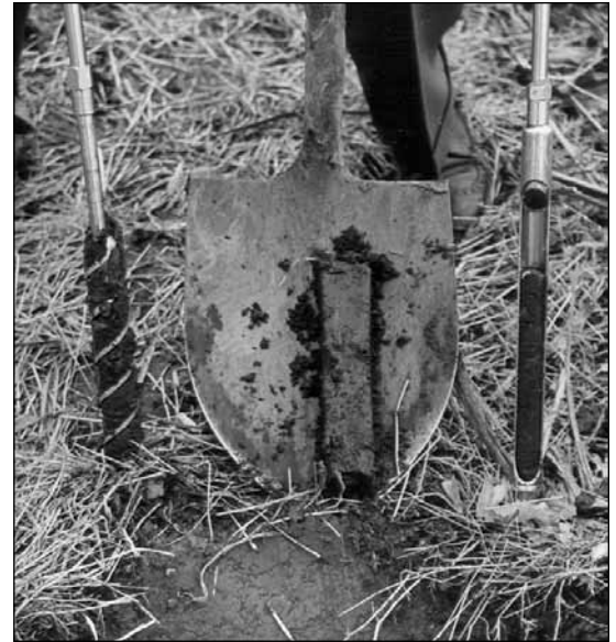
Figure 2. A soil auger (left), spade (center), or probe may be used to sample soils. If you are using a spade, the sample should be trimmed with a knife, as shown.
