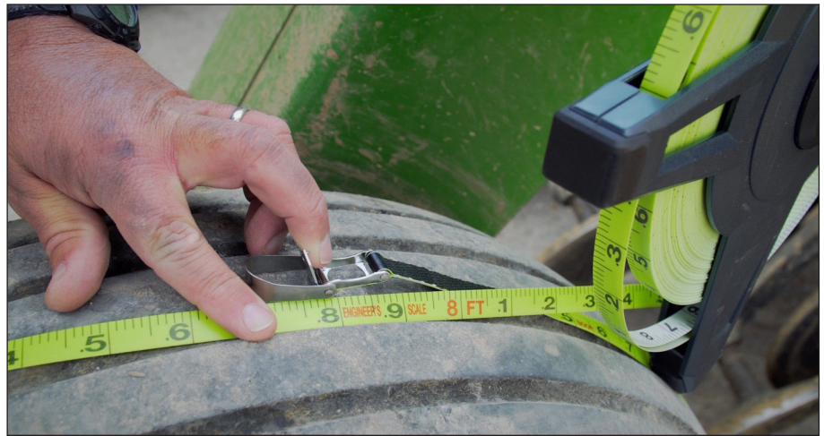
Figure 2. Turn the drive wheel the number of revolutions it would take to travel 150 feet. The number of revolutions can be determined by using the following formula: number of revolutions = 150 feet/circumference of the drive wheel in feet.
