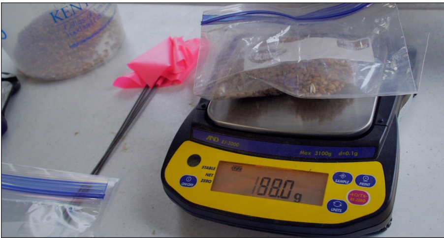
Figure 4. Tare the scale for the weigh container and determine the average weight per disk opener in grams. Compare this weight to the grams of seed/disk opener found in Table 1 for the desired seeding rate and row spacing combination.
