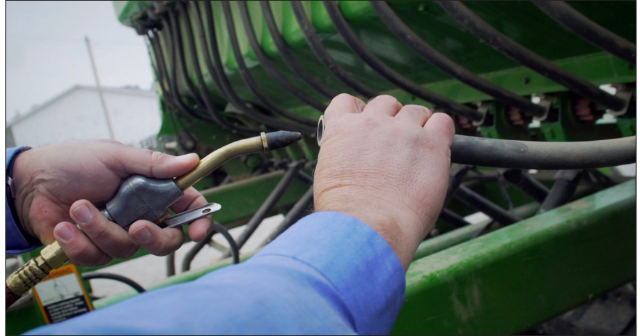
Figure 1. Make sure that seed tubes are clear of obstructions by blowing them out with compressed air.
