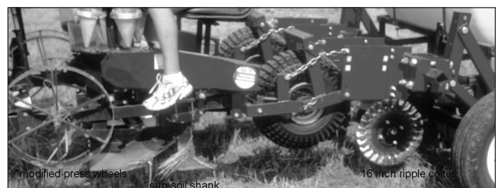
Figure 3. Modifications to a transplanter for no-till transplanting of tobacco.
