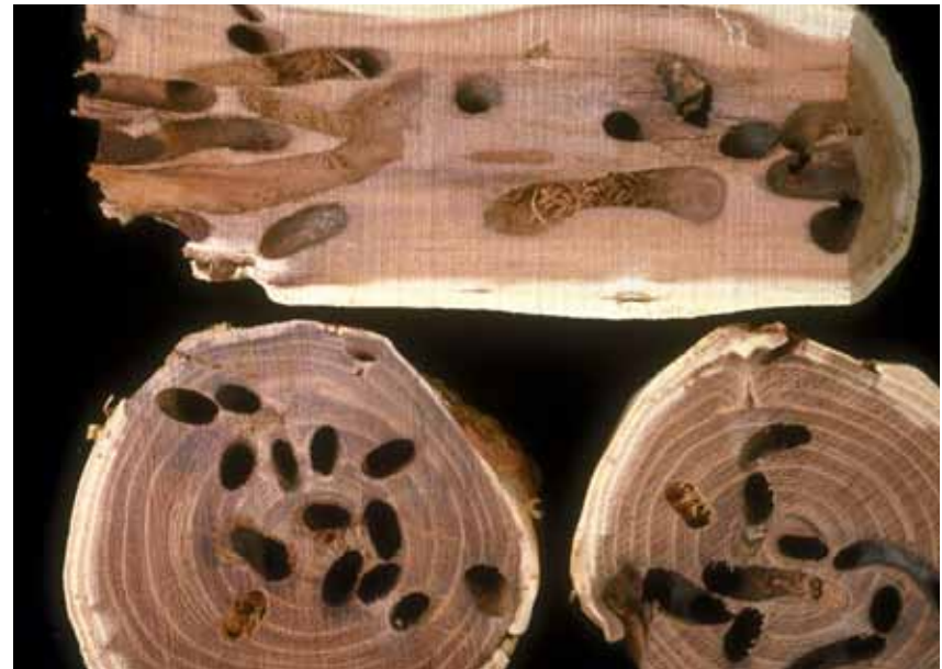
Damaged black locust timber.
