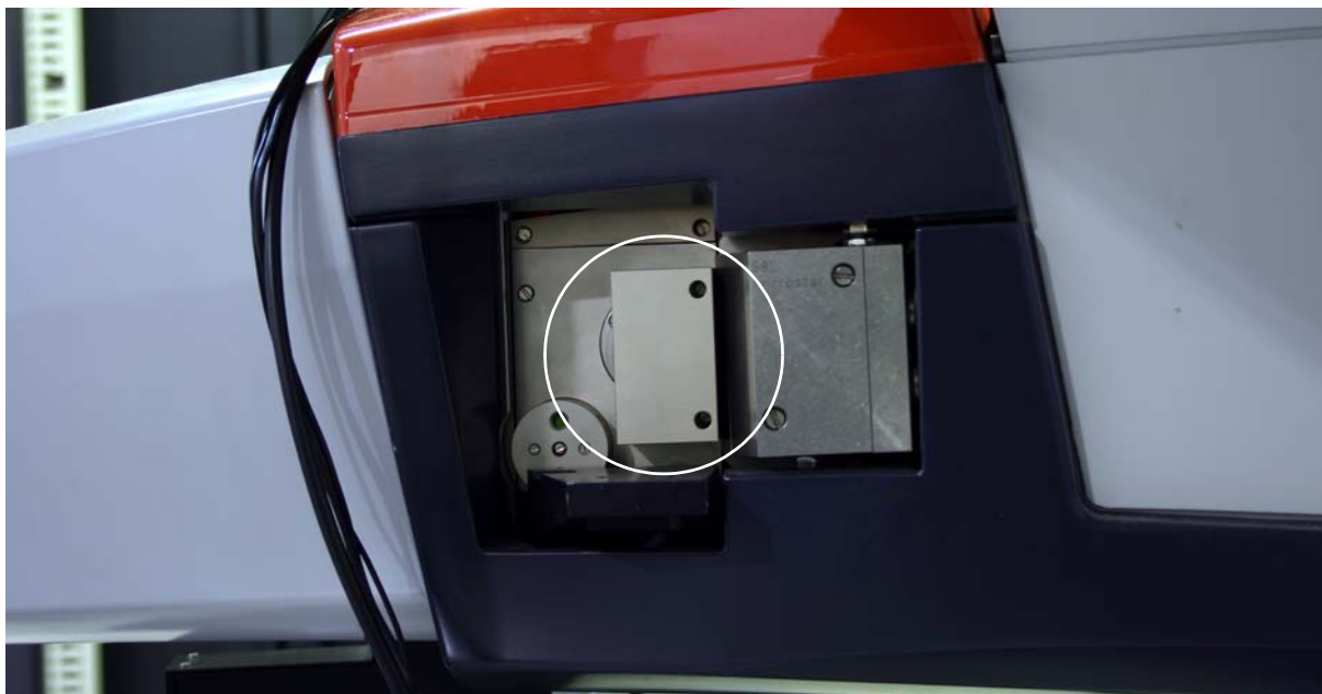
Figure 2.1 – Beam stop block on port
