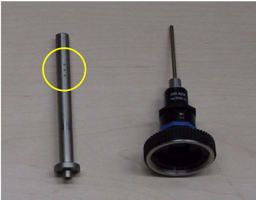
Figure 5.1 — Half-beam alignment pipe (dots circled), half-beam goniometer head tool
