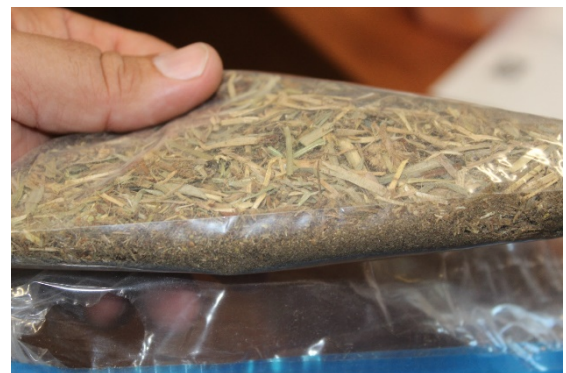
Figure 3. Never subdivide a sample before submitting it to the lab. Core samples are made up of both large and small particles that can segregate making it difficult to get a representative subsample. In this photo the fine particles have move to the bottom of the bag.
