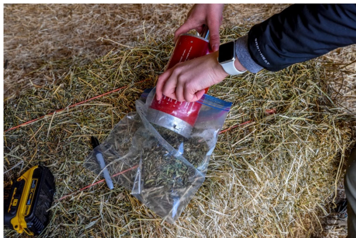
Figure 4. Always submit the entire sample. Subdividing the sample can result in altered lab results since the fine material segregates from the larger particles. Make sure the bag is clearly labeled with all required information.
