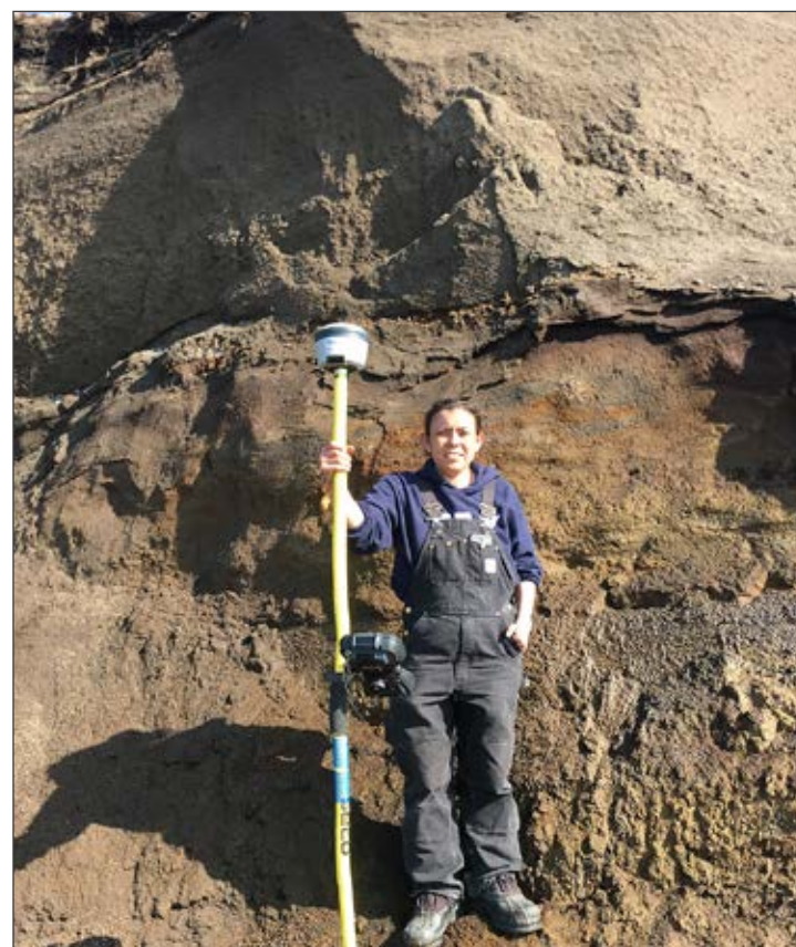
Melissa O'Domin holds a GPS used to measure coastal erosion rates. Photo by Richard Buzard
