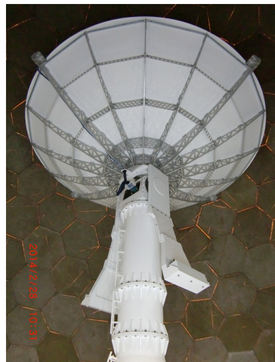
The 8 meters in diameter parabolic antenna inside the radome to observe solar radio wave
