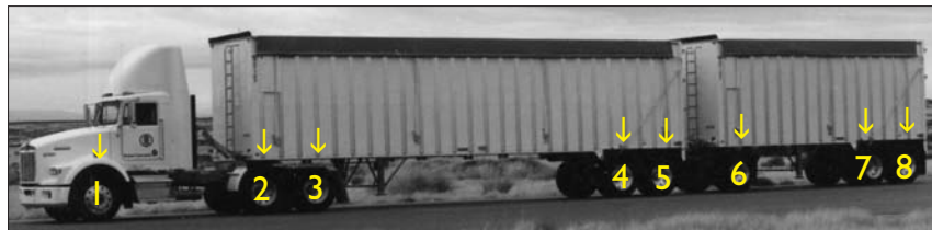
Typical truck configured for 105,500 pounds GVW. (8 axles)
