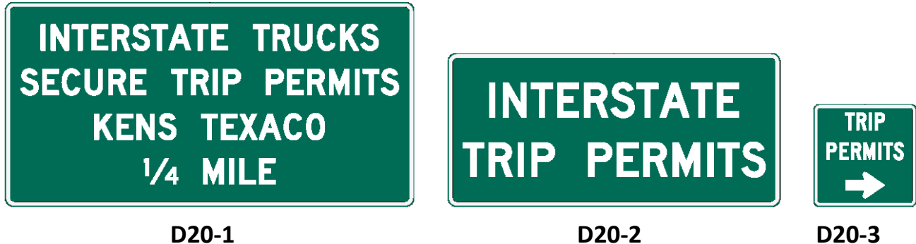
Figure 2D-6 Example Trip Permit Signs
