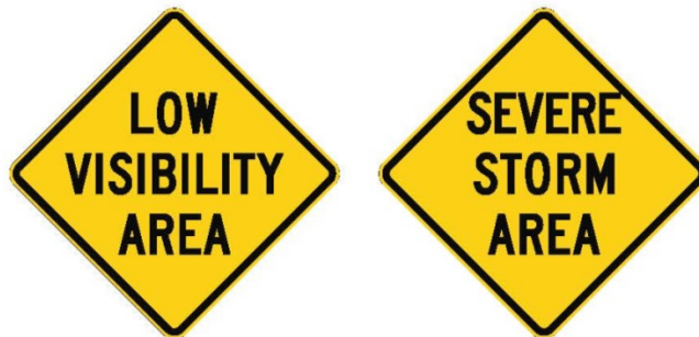
Figure 2C-5 Example Weather Condition Signs
