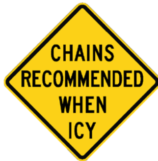
Figure 2C-4 Chains Recommended Sign
