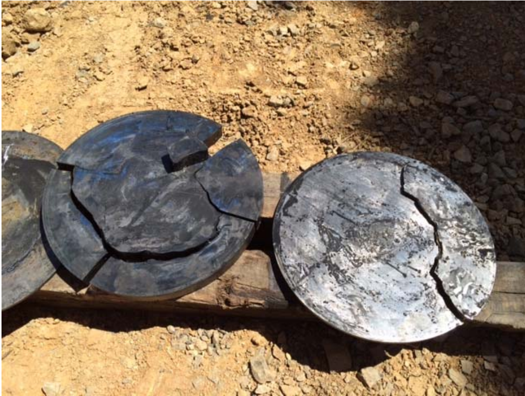
Photo 1. Worn out hammer cushion.
