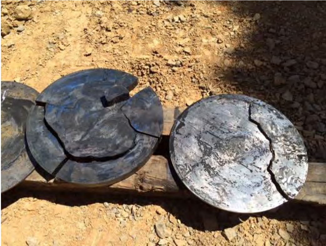
Photo 1. Worn out hammer cushion.
