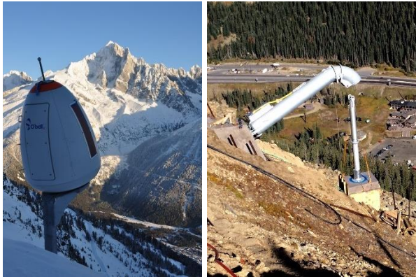
Figure 2: O'Bellx® at Chamonix (left) and Gazex® at 7 Sisters (right, Source: R.Mumford)
