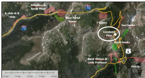
Figure 1: Location of avalanche paths to be studied for Loveland Pass and I-70 (missing Vail Narrows)
