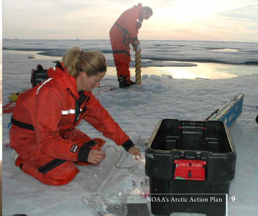
Scientist measures the temperature of a recently drilled ice core. Photo: J. Potter, NOAA.
