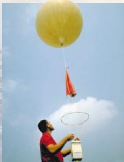
Profiling the atmosphere. A typical network of surface observing stations from which radiosonde balloons (left) collect atmospheric temperature and humidity profiles every 12 hours. An Argo float is the oceanic equivalent of a radiosonde.
