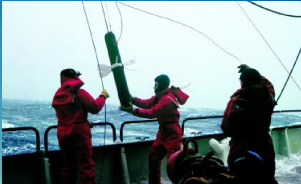
A specially modified profiling float, with propellers to measure vertical currents while it drifts at depth, is lowered into the Labrador Sea in January 1997.
