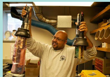
A BGC float sensor head on the left, and a Core Argo one on the right
