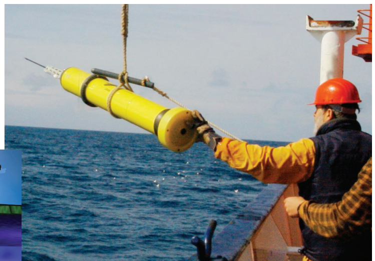
Launching a float (Courtesy of IfM Kiel, Germany)
