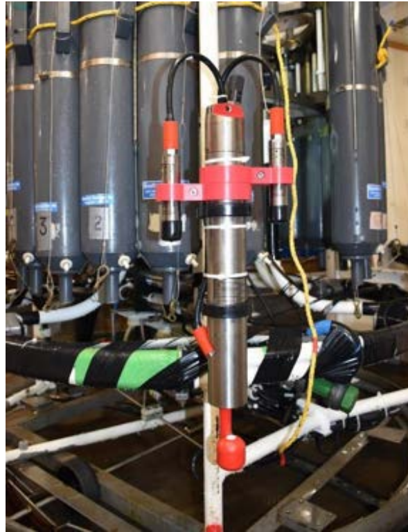
RBR CTD equipped with two RBR dissolved oxygen sensors. Photo: Steve Diggs, SIO.
