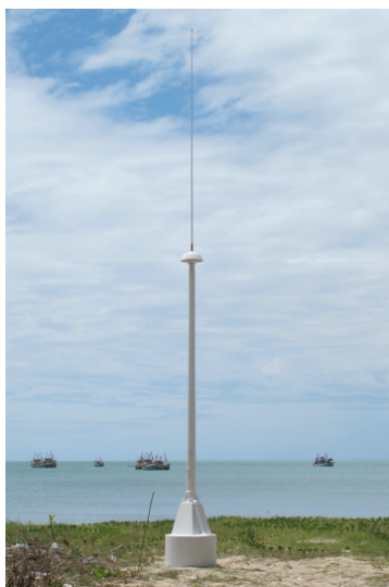
Photo 3: Present-day Coastal Ocean Dynamics Applications Radar (CODAR) having combined transmit and receive antennas in one unit. (Total height is approximately 8 meters for this particular unit).
