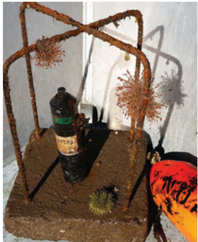
A recovered acoustic telemetry receiver attached to a concrete mooring. The receiver and mooring rest on the estuary or bay substrate with the hydrophone of the receiver pointing upwards toward the surface.
