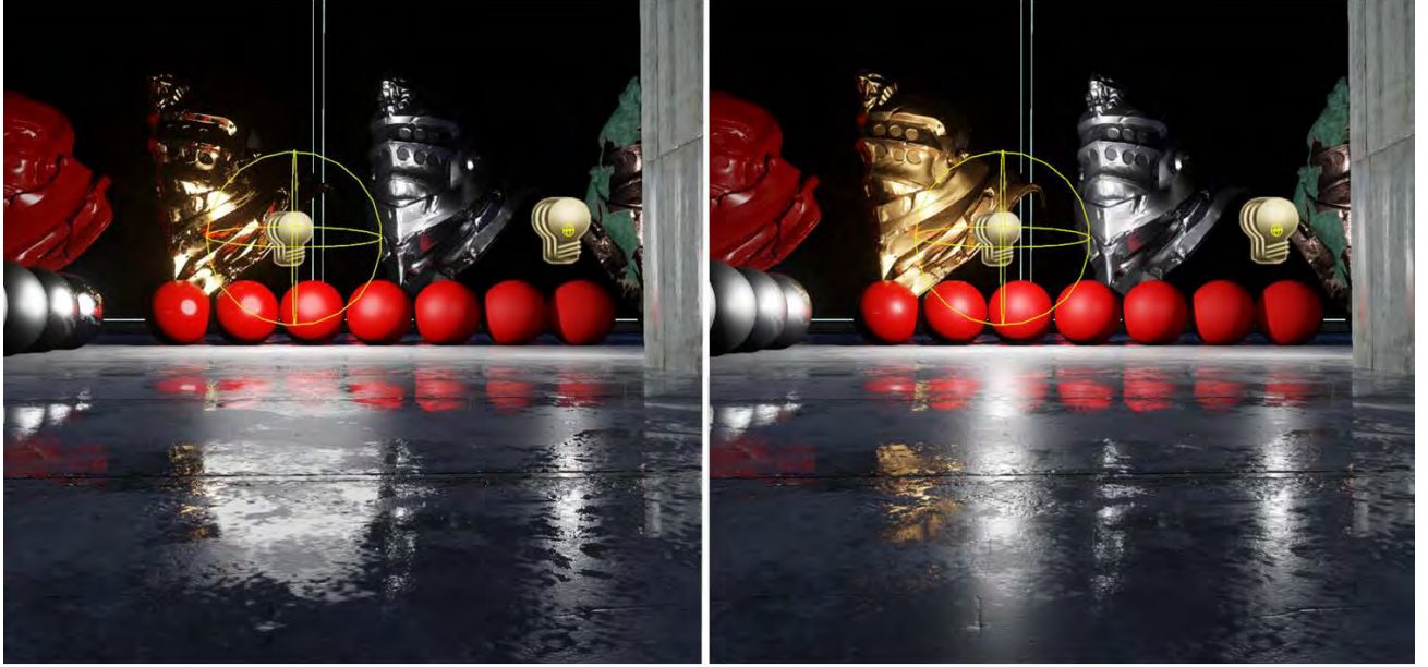
Figure 10: Reference on the left, specular D modification method on the right. The approximation is poor due to the spherical shape getting lost on grazing angles and glossy materials, such as the polished brass head, look rough.
