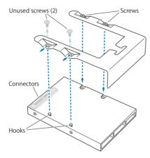
5 Position the drive carrier over the SSD adapter with the drive connectors at the back as shown. Insert the two hooks on the top of the adapter into the carrier's holes. Fasten the two screws on top of the carrier to attach the SSD enclosure to the carrier. 6 Lift the latch and slide the carrier over the guides and into the drive bay until it touches the drive connectors and is seated in the bay.
