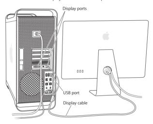
You can connect up to three displays with Mini DisplayPort or Digital Visual Interface (DVI) connectors to the display ports on the back of your Mac Pro. The DVI display port is a dual-link port, so you can connect a 30-inch Apple Cinema HD Display.
