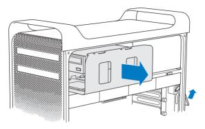
4 Disconnect the cable from the optical drive and remove the carrier from the optical drive bay.
