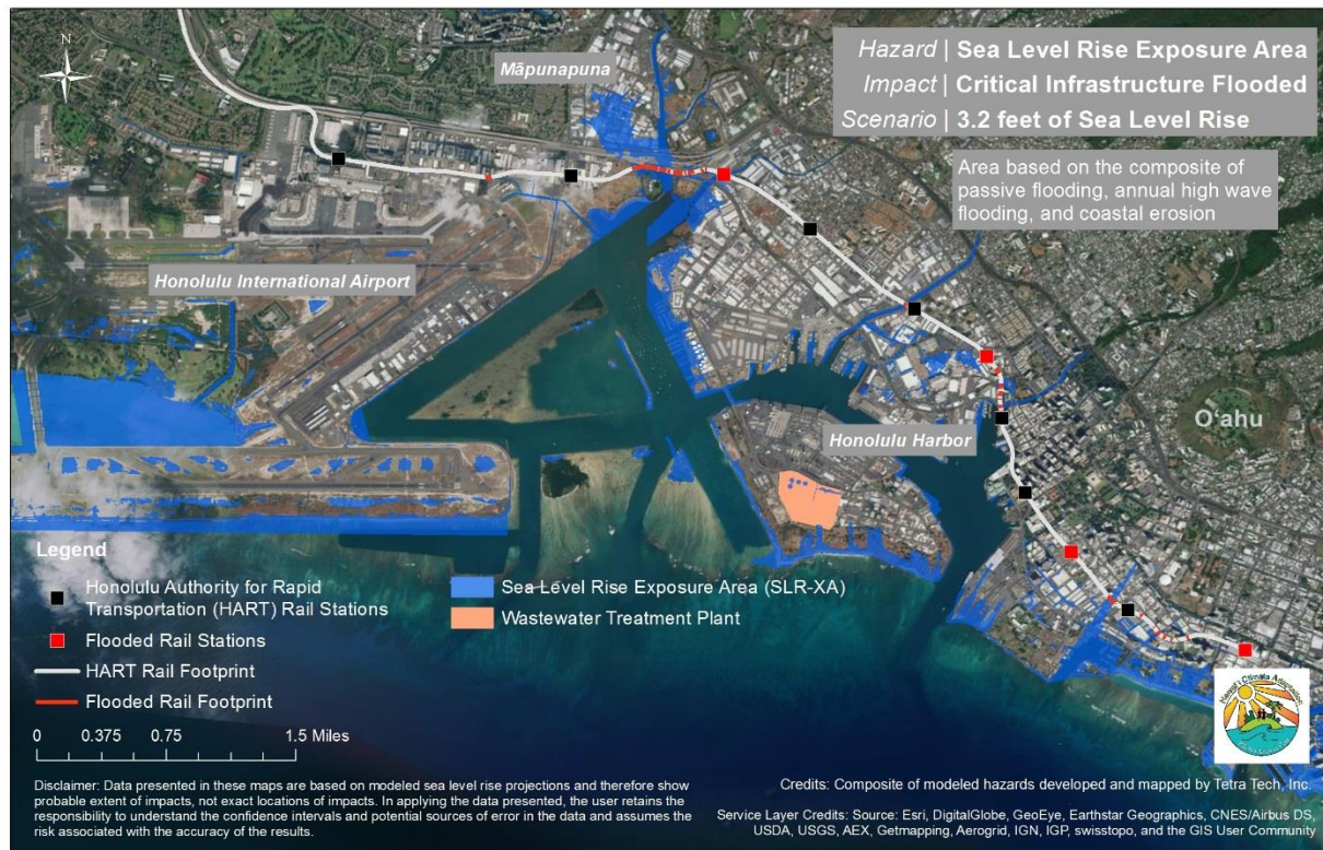
Figure 105. Key transportation facilities and routes in the SLR-XA with 3.2 feet of sea level rise on O’ahu
