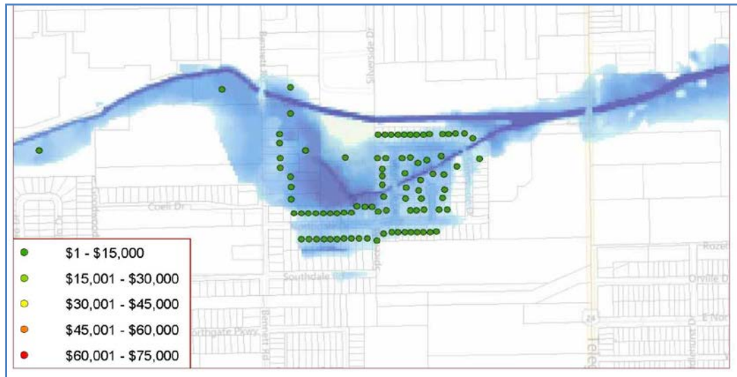
Figure 19. Silver Creek Current Land Use and Current Precipitation 100-year, 24-hour Storm Flooding Damages in One Neighborhood
