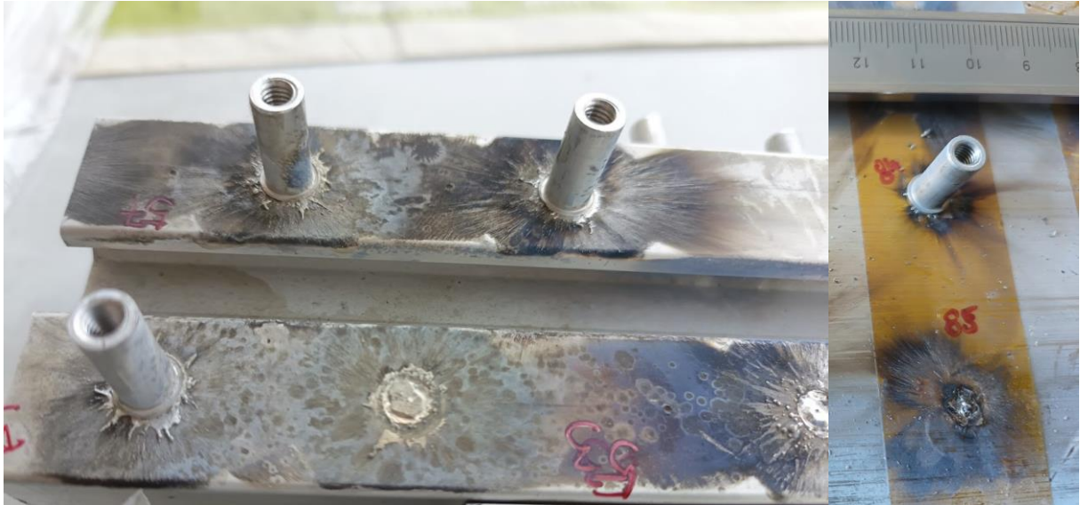
Figure 4.1. This figure illustrates ALMg3 threaded studs joined to an aluminium alloy workpiece with an anodized surface on the left, and a polyimide (Kapton) surface on the right. The surface was pre-penetrated by the impact of a 100 N central hole puncher, simulating the novel impact welding procedure.
