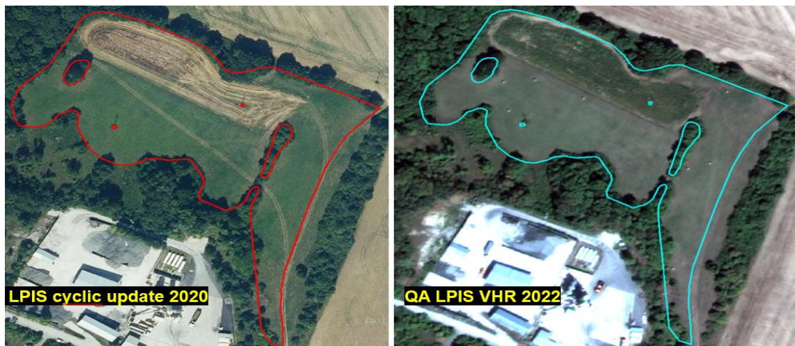
Figure 5.22. Example of the classification error with cause “Erroneous processing “ - a mistake of LPIS operator (part of the LPIS parcel with permanent grassland is used as arable land).
