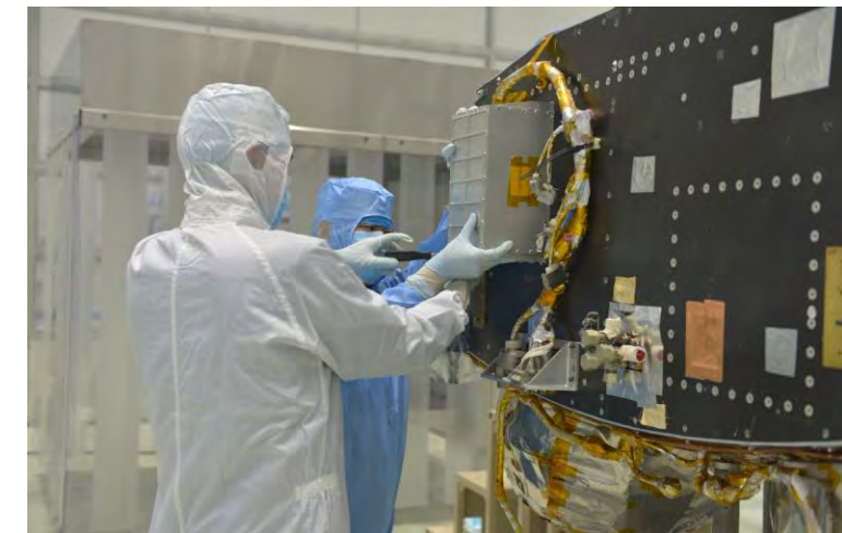
simulated AIT test followed cleanroom operation procedure
