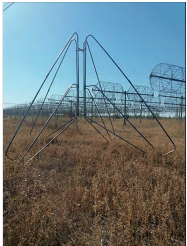
Fig. 1. Active antenna for radio observations at 4—70 MHz. It is cross-shaped and consists of two identical mutually orthogonal symmetric dipoles of a complex shape, mounted on a common holder. The active antenna has also two identical LNAs, each of which is connected to the terminals of the corresponding dipole, from the outputs of which received signals transmitted by electromagnetic waves of two mutually orthogonal linear polarizations are recorded. Such a dipole is identical in shape to any GURT dipole, but all its dimensions have been increased
