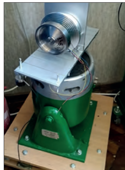
Fig. 3. Testing the reaction wheel on a vibrating stand
