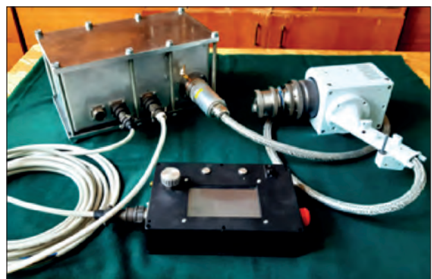
Fig. 3. Complex of hand-held electron beam equipment for technological work in space conditions
