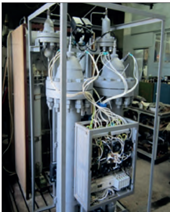
Fig. 5. Laboratory model of hydrogen energy accumulator for this, it is necessary to increase the voltage drop on the electrodes from the current 1—1.5 V to 30—40 V
