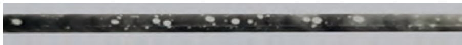
Fig. 4. Roentgenogram of a butt joint of 5456 alloy produced by electron beam welding in the flying laboratory in the mode of reduced gravity of 1/6 g (Lunar surface)
