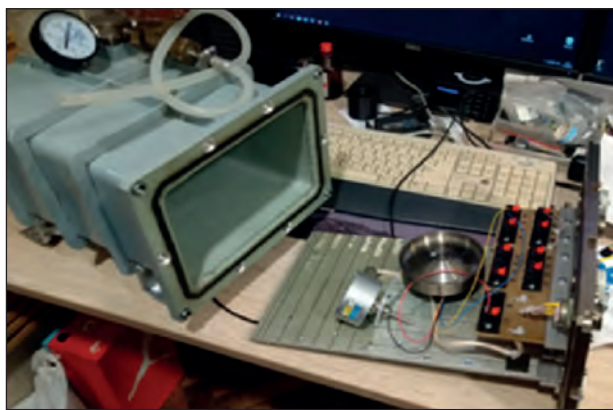
Fig. 5. Checking the reaction wheel parameters
