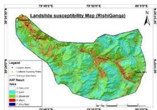
Landslide susceptibility map in parts of Rishi Ganga Valley area region using AHP
