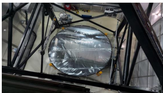
Figure 5: LEFT : Top view of the ILMT showing the liquid mercury mirror covered by a thin mylar film. RIGHT : A panoramic view of 3.6m DOT (left), 1.4m DFOT (middle) and 4-m ILMT facility at Devasthal.
