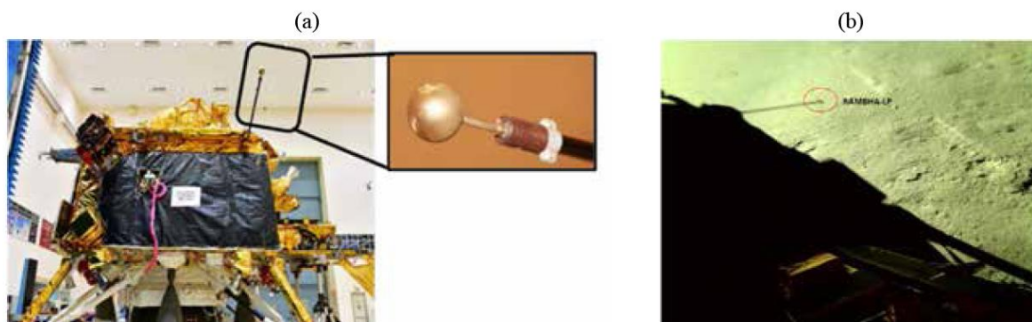
Figure 12: (a) Photograph of RAMBHA-LP system during Spacecraft level Deployment & Functional Test. (b) The photograph the Chandrayaan-3 lander, showing the shadow of the deployed LP.
