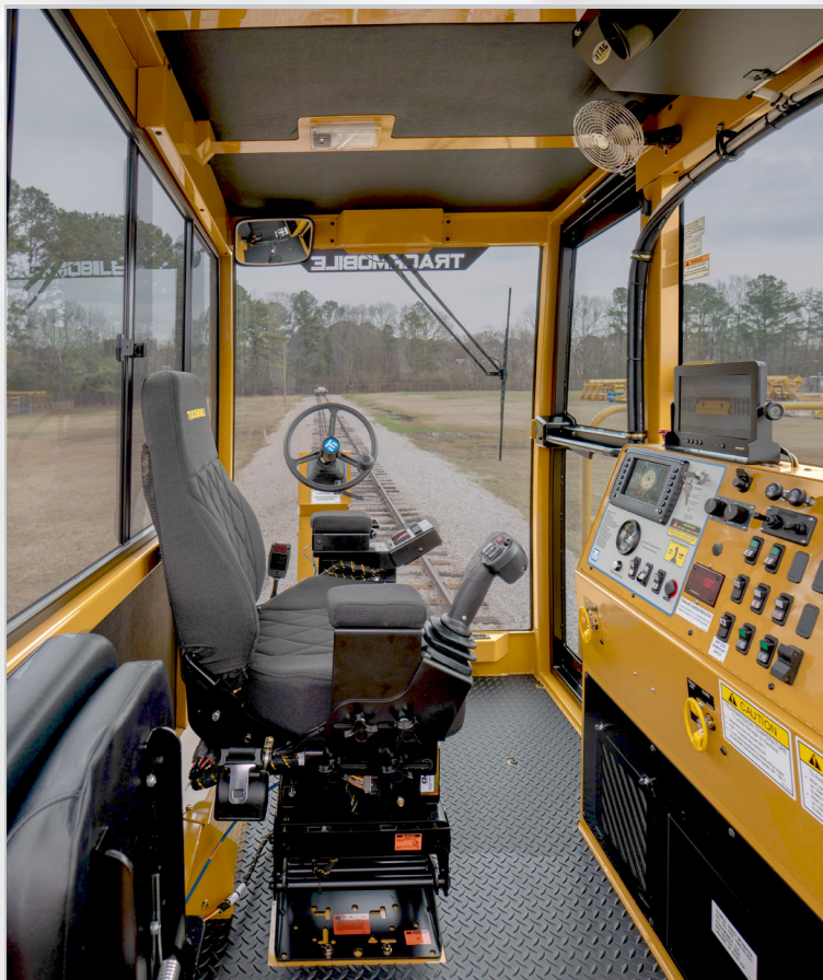
Atlas control panel and operational controls.
