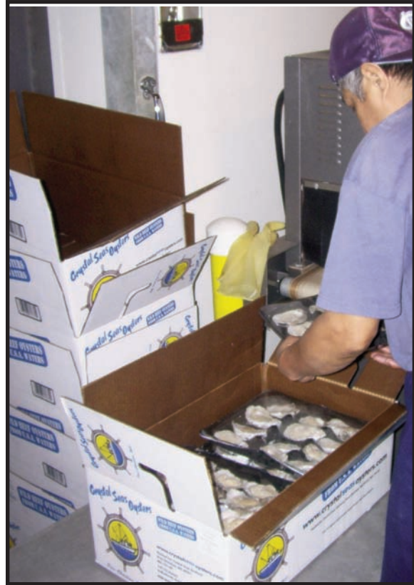
Individually quick-frozen (IQF) oysters in covered plastic trays are being boxed at the postharvest processing (PHP) plant in Pass Christian by oyster PHP dealer Crystal Seas Seafood. IQF oysters are made to pass through nitrogen or carbon dioxide tunnels for freezing. These oysters are processed to deliver quality of product, increased shelf life, taste, convenience and peace of mind on food safety.
