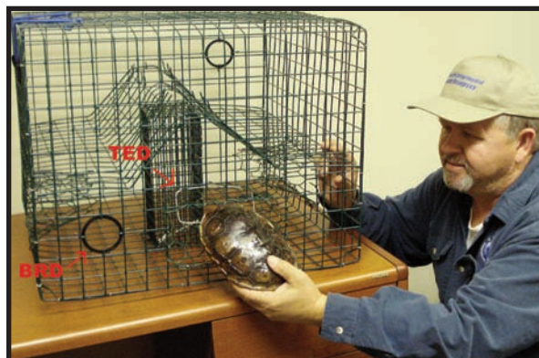
Fisheries Technician Rudy Balias shows how new TED-equipped crab traps prevent terrapin capture.
