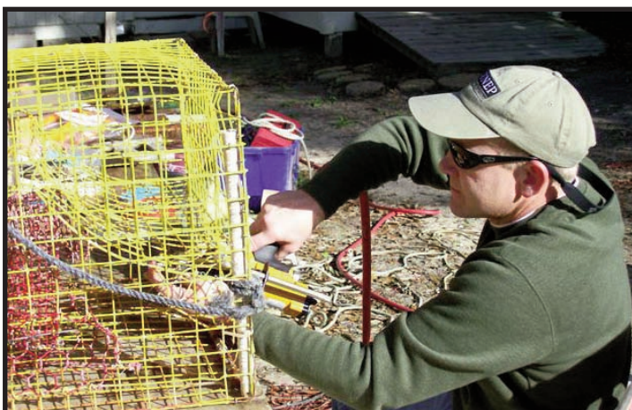
Fisheries Projects Officer Darrin Stewart installs Diamondback Terrapin Excluder Devices (TEDs) in the traps of a commercial crab fisherman.
