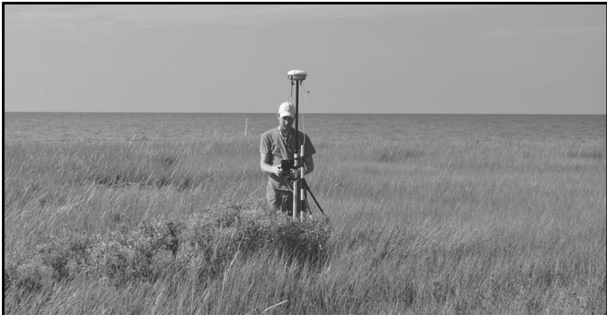
Grand Bay National Estuarine Research Reserve scientist Tom Strange uses survey equipment to measure erosion rates at the reserve.
