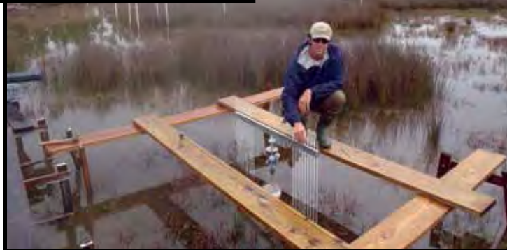
NERR staff measuring subsidence and accretion of marsh elevation at NERR, part of a broader sentinel site program to measure impacts of sea level rise in our nation's estuaries.
