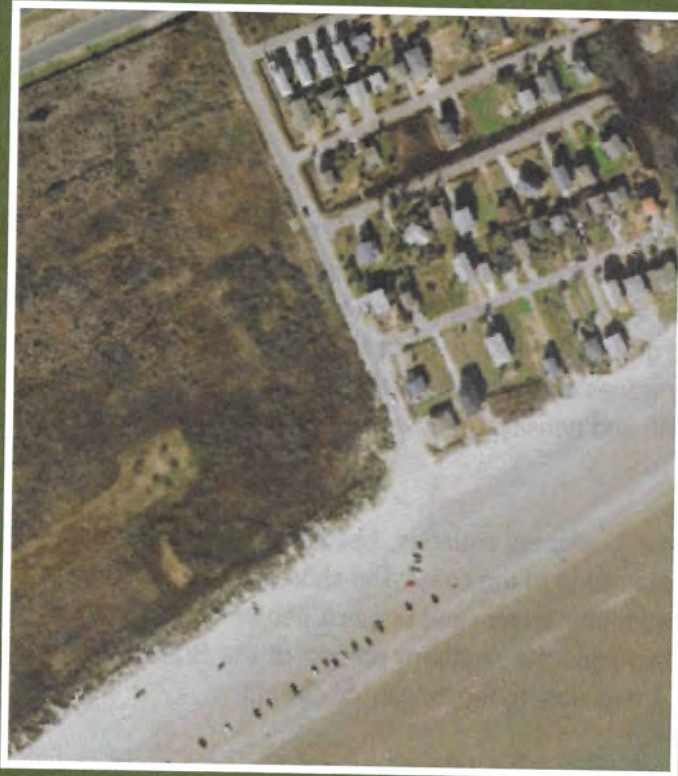
Figure 8. Aerial imagery of natural dune formation adjacent to shorefront development on Galveston Island. Natural dunes exist where there is room for dunes to migrate.
