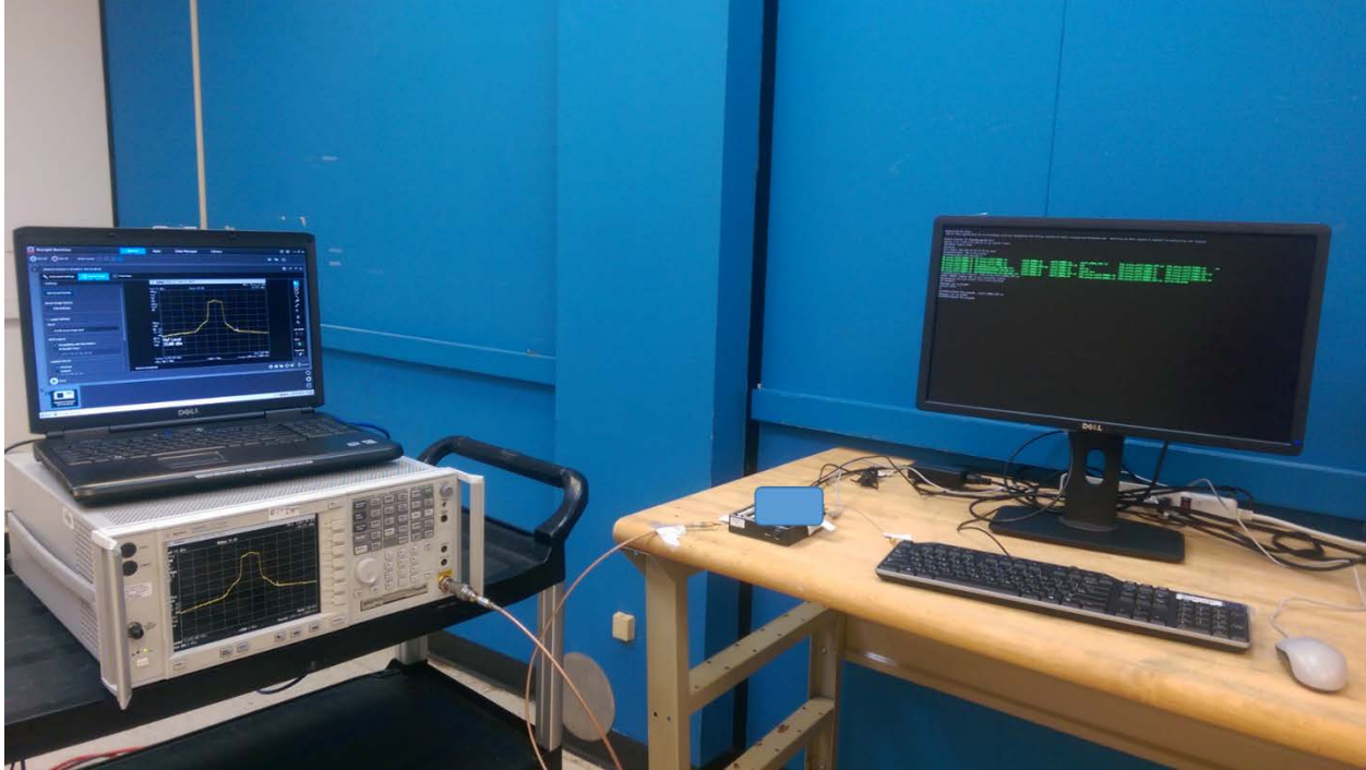
Figure 212 – RF Characterization test setup
