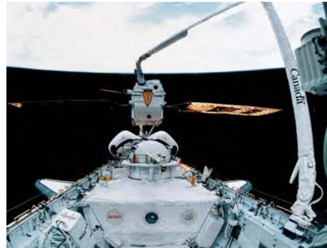
Eureca's solar wings were safely deployed before the free-flyer was released. (NASA)
