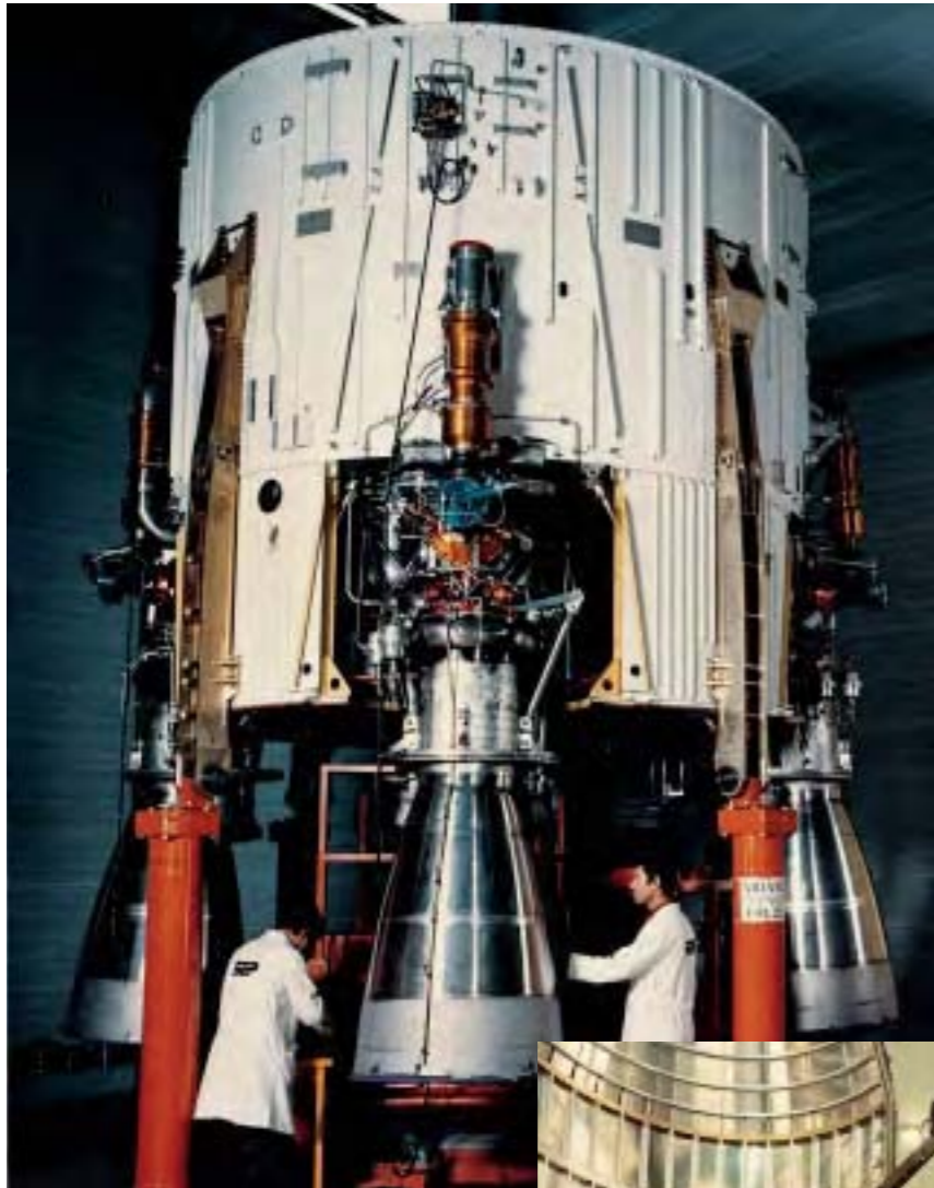
The engine bay of Ariane's first stage carried four Viking 5 engines. (Sneema Moteurs)
