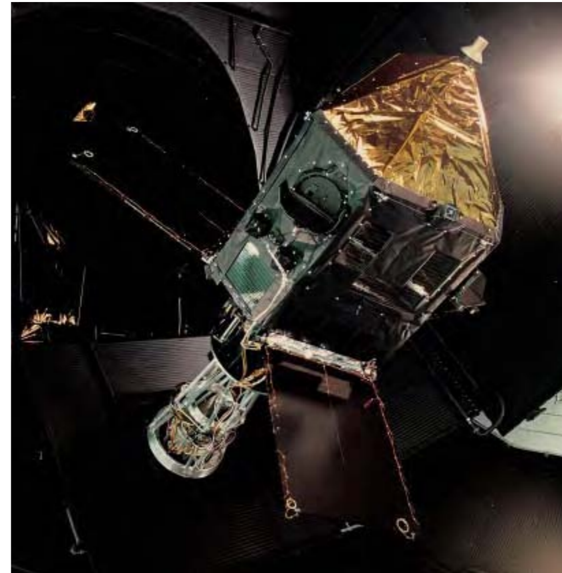
Hipparcos final qualification testing in the Large Space Simulator at ESTEC. One of the telescope's two semi-circular apertures is seen closed; the other is side-on at far right.
