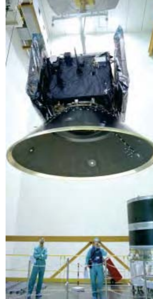
SMART-1 is hoisted towards installation on its Ariane-5 launch vehicle. (ESA/CSG)
