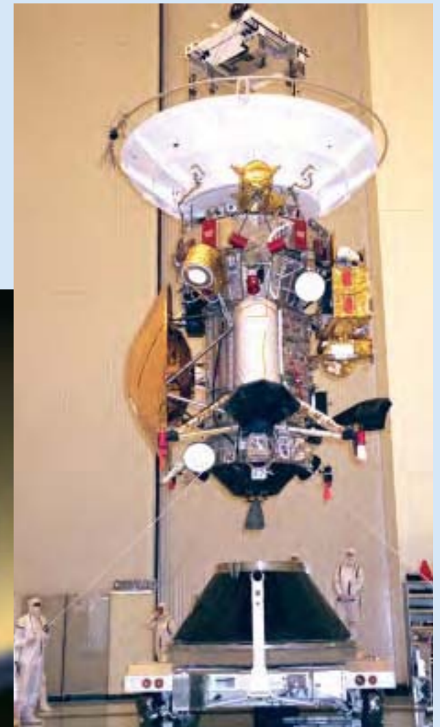
Cassini, with Huygens mounted on the side, is lowered on to its launch vehicle adapter in the Payload Hazardous Servicing Facility at the Kennedy Space Center. The Huygens Engineering Model is in the Huygens Probe Operations Centre (HPOC) at ESOC, used as a testbed during the cruise to Saturn. (NASA)
