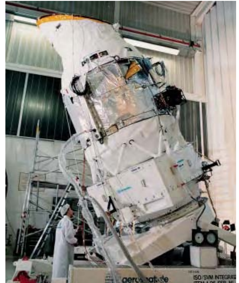
ISO's payload module was supported by the service module below. (Aerospatiale)
