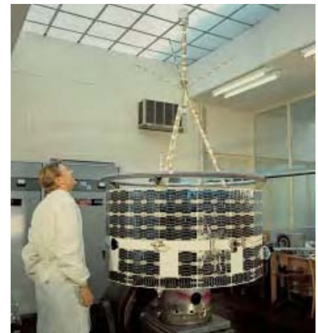
HEOS' 1.7 m boom held the magnetometer away from the body's magnetic influence. HEOS-2 (seen here) was similar to its predecessor but notably carried a loop antenna just above its main body for solar radio observations.
