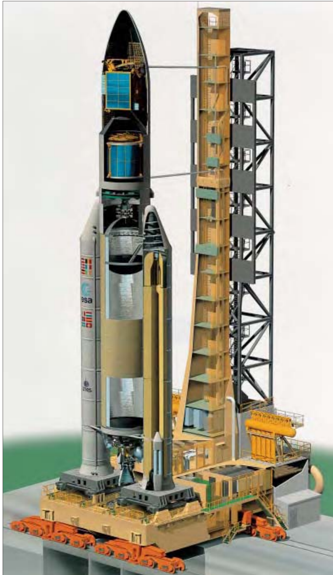
Cutaway of the Ariane-5G vehicle on the ELA-3 launch pad. (ESA/D. Ducros)
