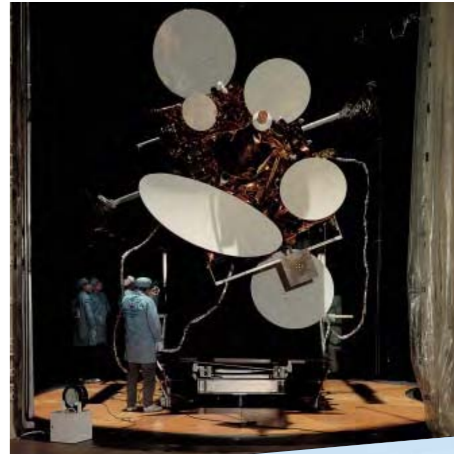
Olympus undergoing electromagnetic compatibility testing at the David Florida Laboratory in Canada.
