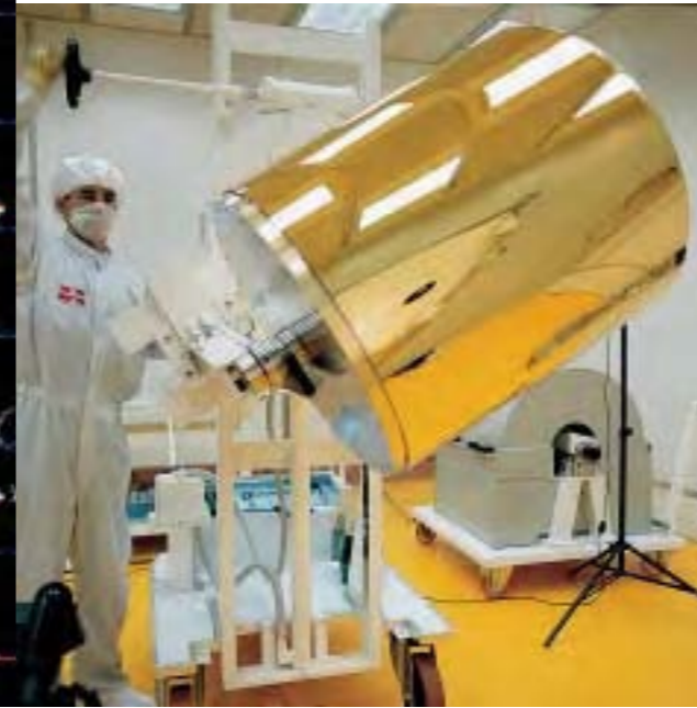
Right: each of XMM's mirror modules houses 58 nested mirrors to reflect the incoming X-rays to a focus. Two modules also have a grating stack for spectroscopy.
