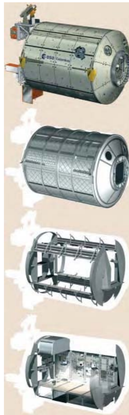
The layers of Columbus. From top: complete with Meteoroid & Debris Protection System; the primary pressure vessel; the secondary structure; the payload racks. (ESA/D. Ducros)
