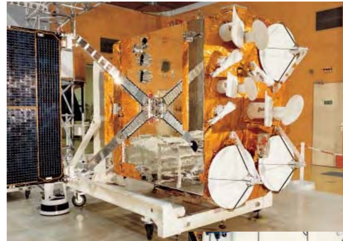
ECS-2 and subsequent satellites reconfigured the antenna platform, adding the Satellite Multiservice System for business data transmissions.
