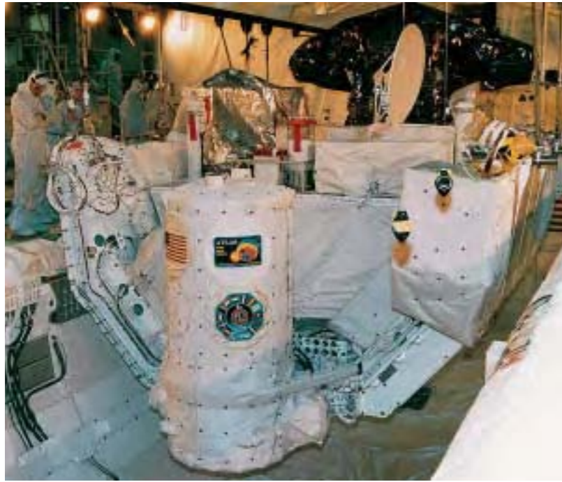
The Atlas Spacelab missions did not include a Pressure Module, but instead housed the avionics in an Igloo (foreground) for controlling the payloads on the two Pallets. (NASA)
