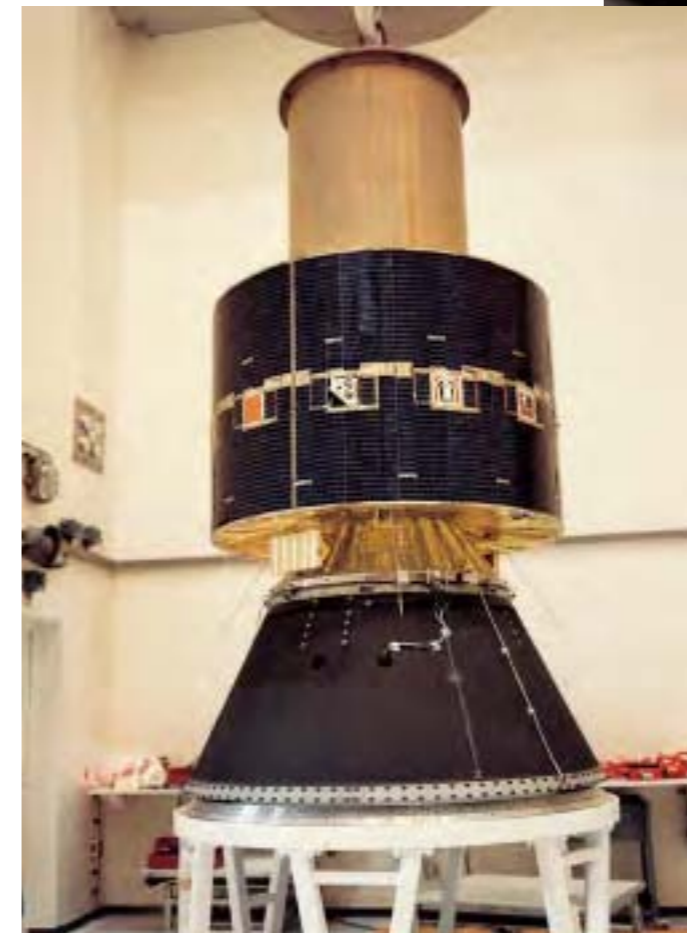
Sirio-2 ready at Kourou for encapsulation in the Ariane payload fairing. The despun antenna is covered by a protective cylinder (top). (ESA/CNES/CSG)
