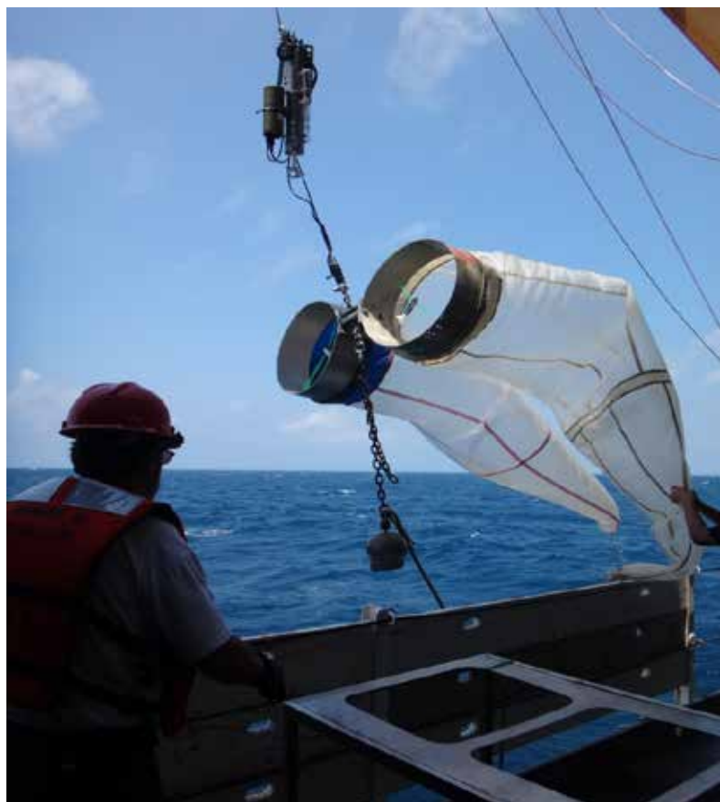
Figure 10-5 Photograph of bongo net being deployed with Seacat CTD on the wire above bongo
