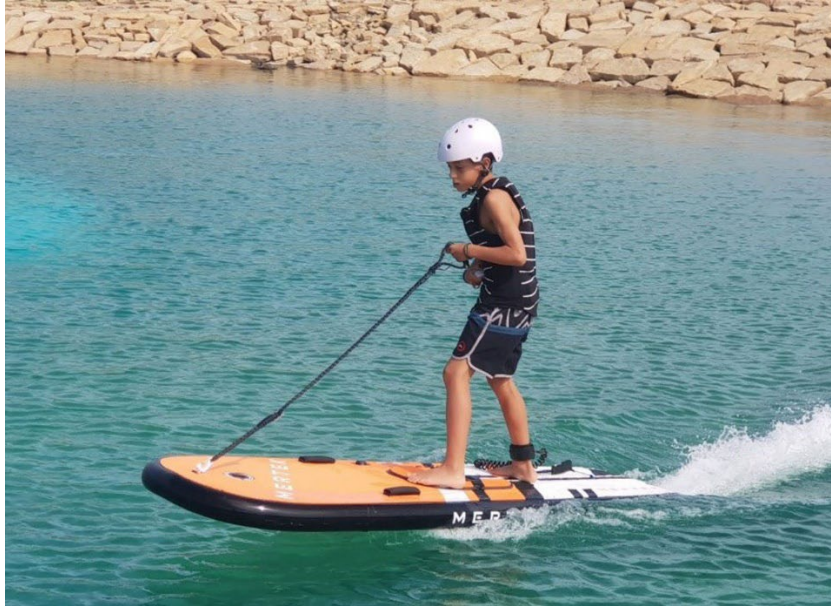
Mechanically Propelled Surfboard (MPS)- also known as a jet board, is a vessel that consists of a board using a surfboard-type design fitted with propulsion machinery (either electric or internal combustion).
