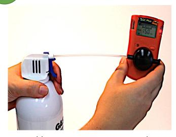
Aerosol bump test may not reach target concentration (25 ppm) using the aerosol spray method
