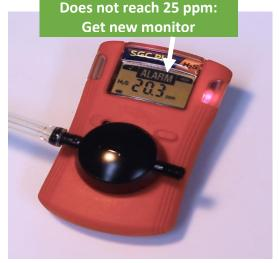
Aerosol bump test may not reach target concentration (25 ppm) using the aerosol spray method **Do not use monitor if**:
