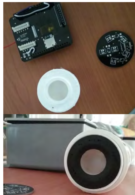
Fig. 3. Components and assembled optical sensor.
